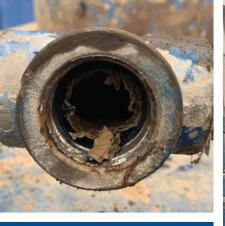
By installing a gauge at every cylinder, you can detect clogs in the line before it becomes a problem.
